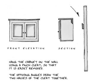
The basic principle involved is to lock together two boards cut at an angle. The piece will be hung securely from the top, as long as no one pushes up on it and disengages the cleat. When hanging, the bottom of the cabinet presses hard against the wall, which is why the hanging surface must be sturdy and rigid. There are lots of fun ways to use this technique on different types of scenery. It is great for quick assemblies.
